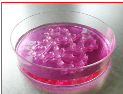
Figure 5: Square arrangement of filter spacers offers proper contact face for filter paper
