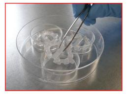
1. Place three small petri dishes in one large petri dish and insert one filter spacer into each small petri dish ensuring correct positioning of filter spacer with <u>pin</u> <u>orientation upwards!</u> (See figure 2.)
