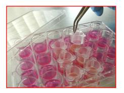
*Figure 7:* Remove the transport protectors, preventing skin models from damaging during transportation.
